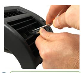
Push front of tab while pulling on back of tab. Tab will slide together and lock onto the louver.
